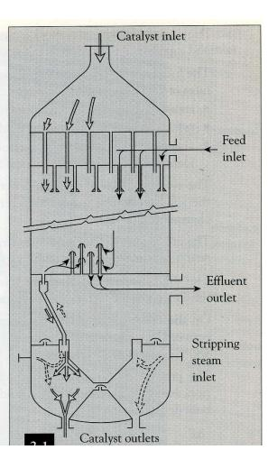
If the speed passage of the gas into the channel becomes excessive, this causes the antrainment of the solid with the reactor effluent. To prevent this situation, it is mantain this speed limit beyond a certain limit.
