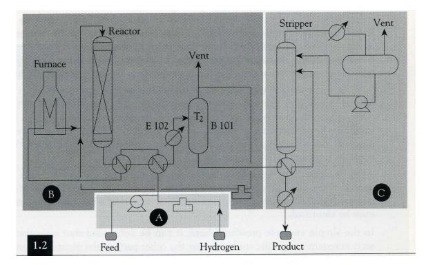
This system can be divided into three indipendent subsystem. System B, which includes a recycle, CAN NOT BE BROKEN DOWN FURTHER and it contains several parts with disctint functions. IT CAN BE DESCRIBED BY A COMPLEX MODEL. The models of sub-systems A and C are simple. These definitions are not very rigorouses.
